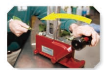
1. Pull handle forward to advance pick
