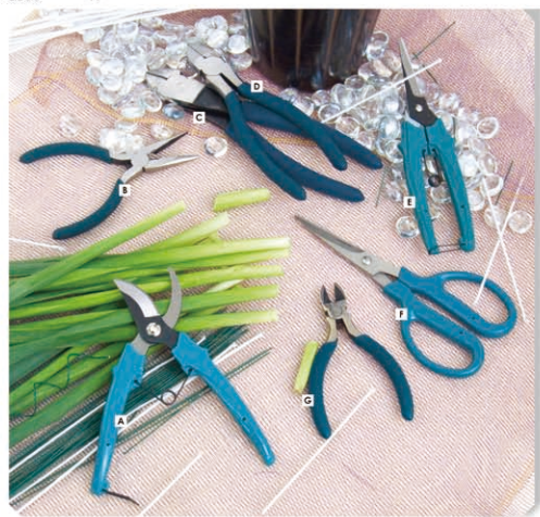
Items depicted from opposite page: A. Secateurs, B. Needle Nosed Cutters, C. 8" Cutter, D. 6" Cutter, E. Shears, F. Scissors, G. 4.5" Diagonal Wire Cutters.
