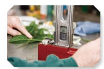
2. Insert stem into jaws - push handle away to close pick around stem
